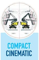
With it special railway design, the Delta boom makes possible to bypass the obstacle made by the contact line and allows to open the complete kinematics of the boom without restriction.
