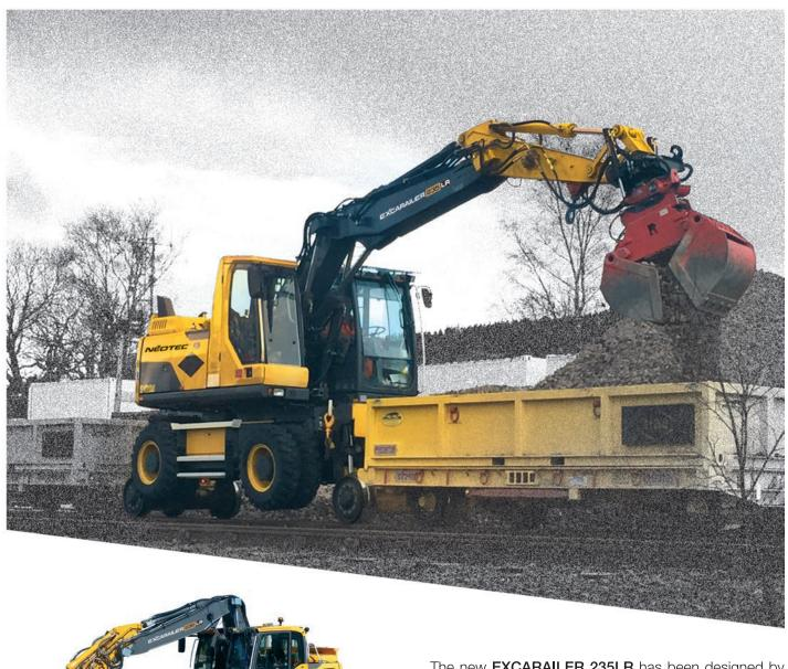
The new **EXCARAILER 235LR** has been designed by NEOTEC in co-operation with Volvo Equipment based on their 150E. This Roadrail Excavator meets the requirements of the most demanding railway construction and renewal works while preserving the best stability and compactness in its class. The two-cab design offers the best in term of comfort and safety.
